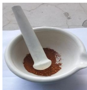
Figure 1(e) Photograph of the top-view of as-prepared powder of iron concretion
