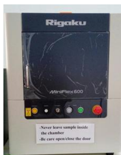
Figure 2 photograph of X-ray diffractometers
